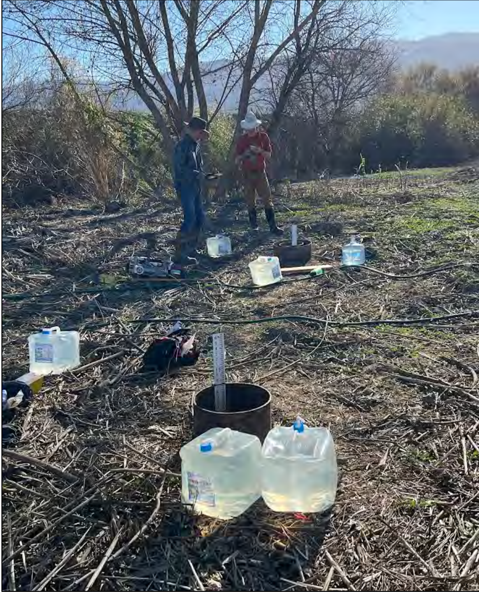
Figure 10. Single-ring and double-ring infiltrometer tests downstream of Bend #1 on January 15, 2025, Somavia Reach of Salinas River, Chualar, Monterey County, CA. The single-ring infiltrometer was 16 inches diameter, and the double-ring infiltrometer was 12 inches and 20 inches diameter.
