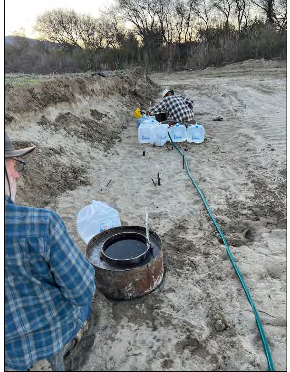
Figure 10. Single-ring and double-ring infiltrometer tests downstream of Bend #1 on January 15, 2025, Somavia Reach of Salinas River, Chualar, Monterey County, CA. The single-ring infiltrometer was 16 inches diameter, and the double-ring infiltrometer was 12 inches and 20 inches diameter.
