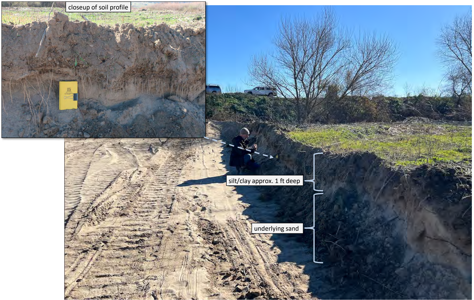
Figure 8. Example alluvial deposits found at the downstream of Bend #1 site, Somavia Reach of Salinas River, Chualar, Monterey County, CA. A silt-clay of about one foot in depth overlying fine to medium alluvial sand.
