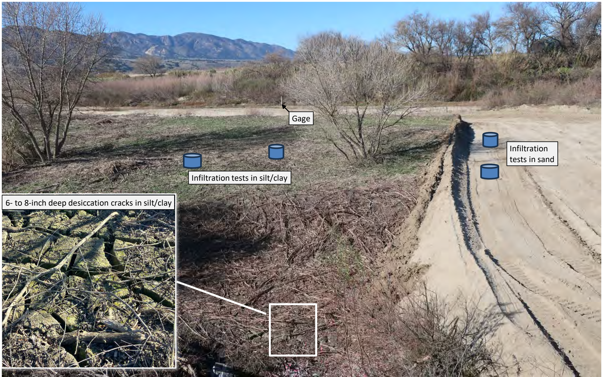
Figure 9. Soil infiltration test sites conducted downstream of Bend #1 on January 15, 2025, Somavia Reach of Salinas River, Chualar, Monterey County, CA. 6- to 8-inch deep desiccation cracks were found in alternate-channel silt-clay deposits but not on the upper overbank surface.
