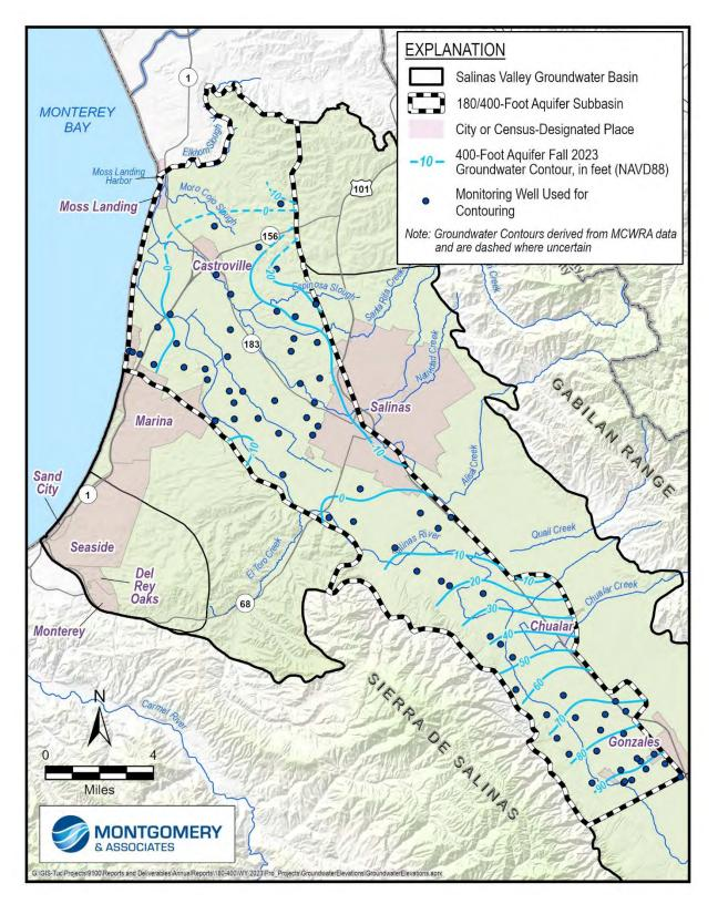
Figure 3-20. Fall 2023 Groundwater Elevation Contour Map for 400-Foot Aquifer
