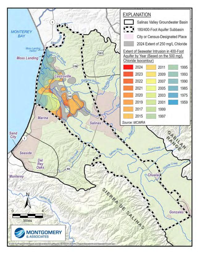
Figure 3-17. Seawater Intrusion Contours for the 400-Foot Aquifer
