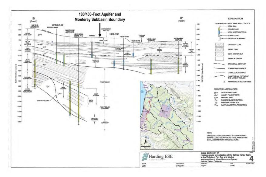
Figure 3. Cross Section of SVA and Intermediate Aquitard (adapted from Harding ESE, 2001)
