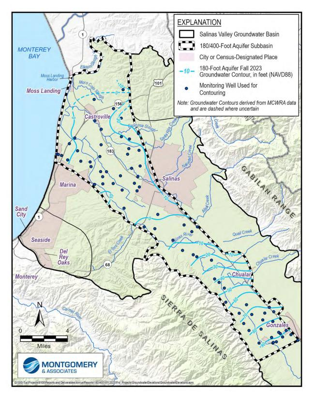
Figure 3-18. Fall 2023 Groundwater Elevation Contour Map for 180-Foot Aquifer
