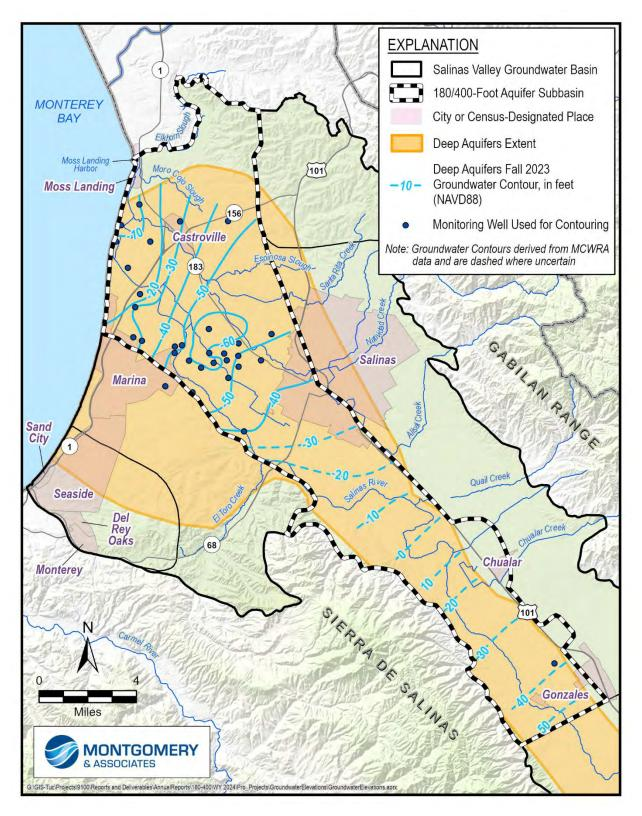
Figure 3-22. Fall 2023 Groundwater Elevation Contour Map for Deep Aquifers
