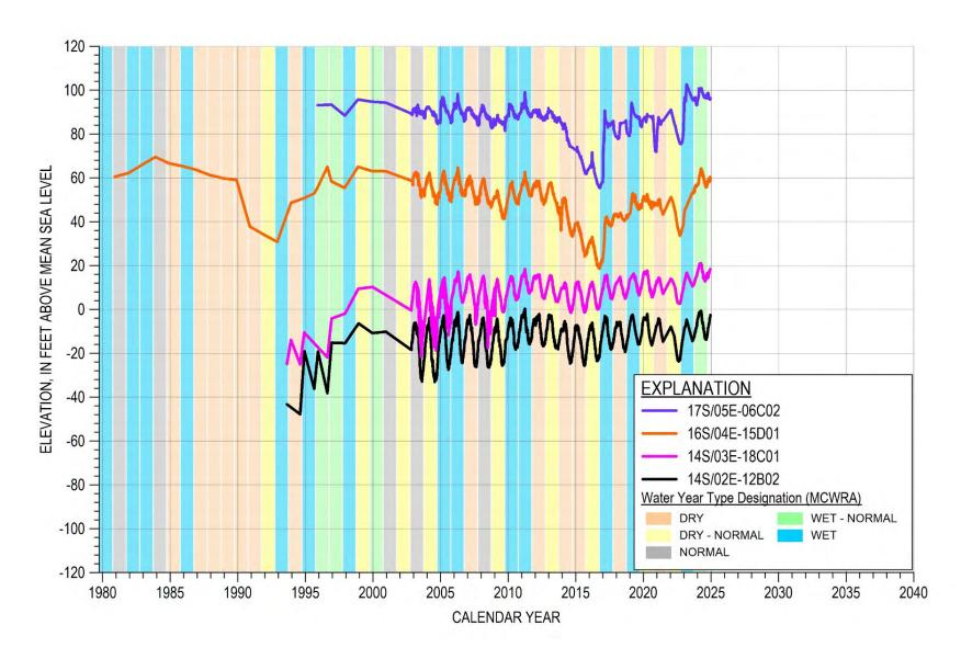
Figure 3-13. Groundwater Elevation Hydrographs for Selected Monitoring Wells in 180-Foot Aquifer
