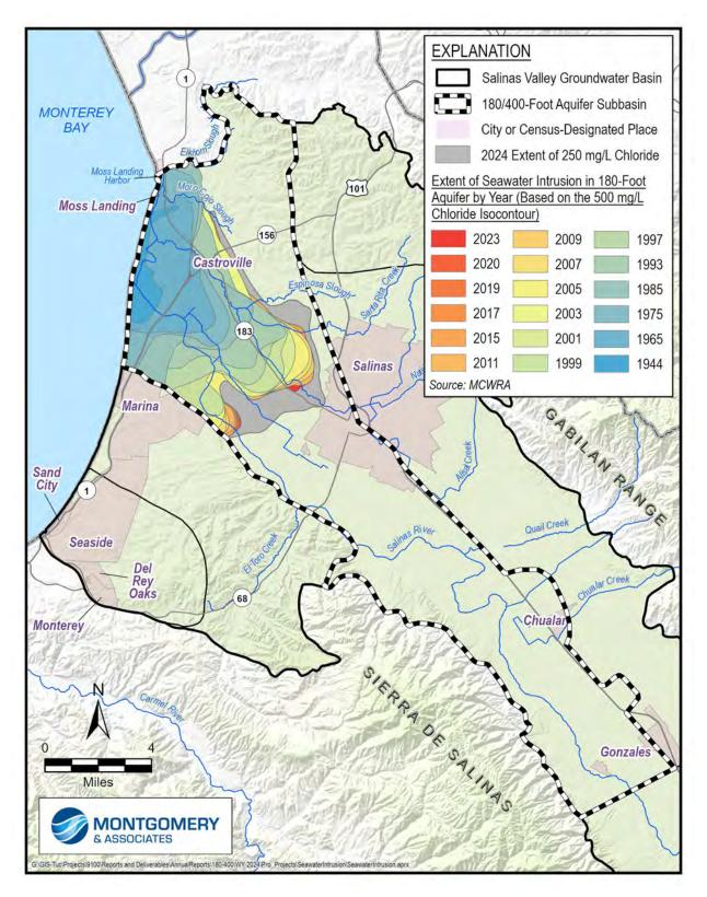
Figure 3-16. Seawater Intrusion Contours for the 180-Foot Aquifer
