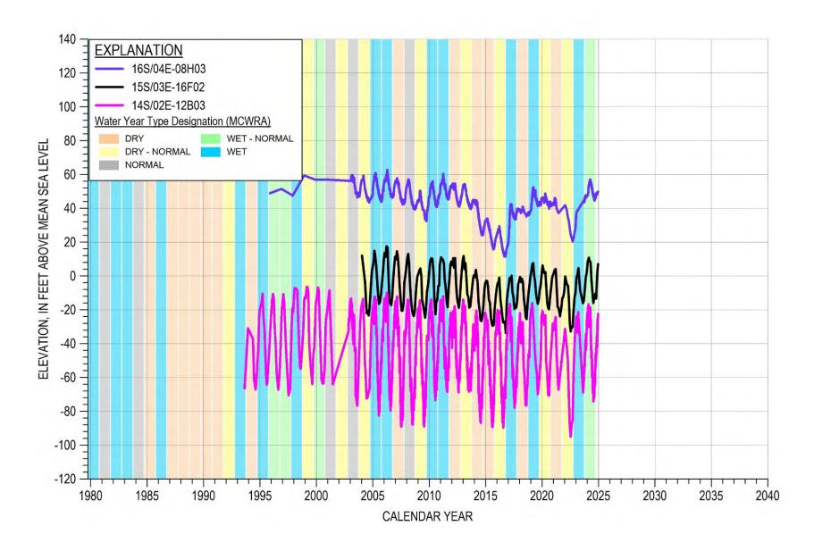
Figure 3-14. Groundwater Elevation Hydrographs for Selected Monitoring Wells in 400-Foot Aquifer
