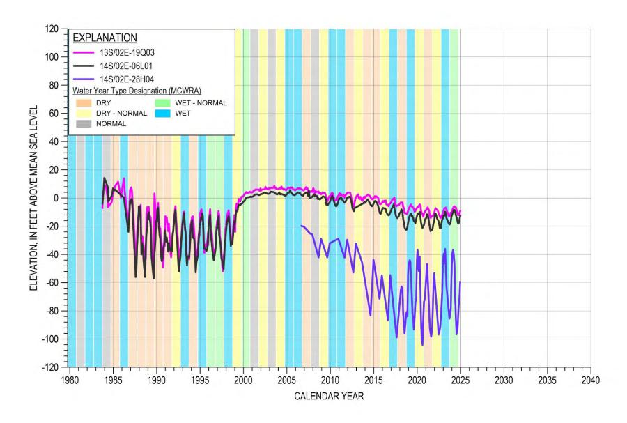
Figure 3-15. Groundwater Elevation Hydrograph for Selected Monitoring Well in Deep Aquifers
