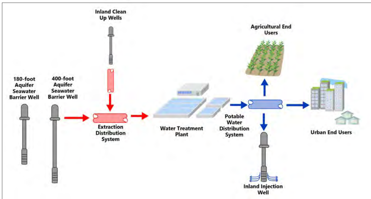
Figure 5. Components of Brackish Groundwater Restoration Project
