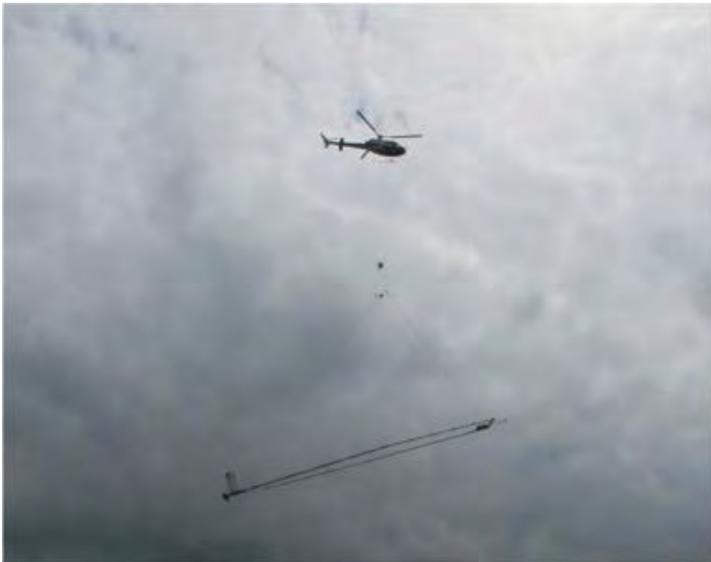
Figure 3 SkyTEM312HPM Airborne unit.
