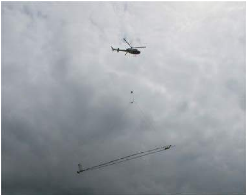
Figure 3 SkyTEM312HPM Airborne unit.
