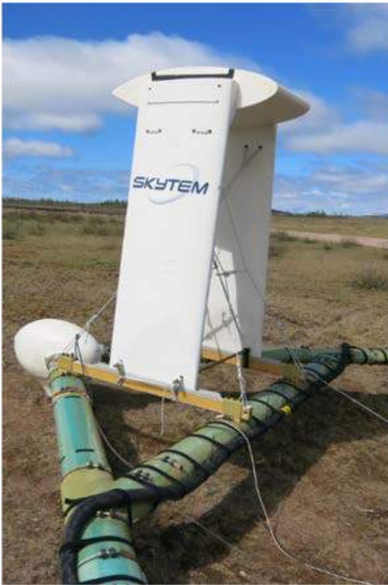
Figure 5 Rudder containing the Z coil located in the top part of the tower.
