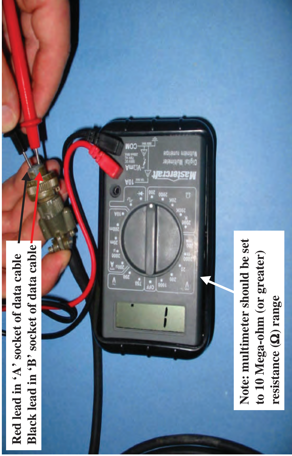
Pic.11 Test wireline 'A-B' resistance at data cable (should be off-scale)
