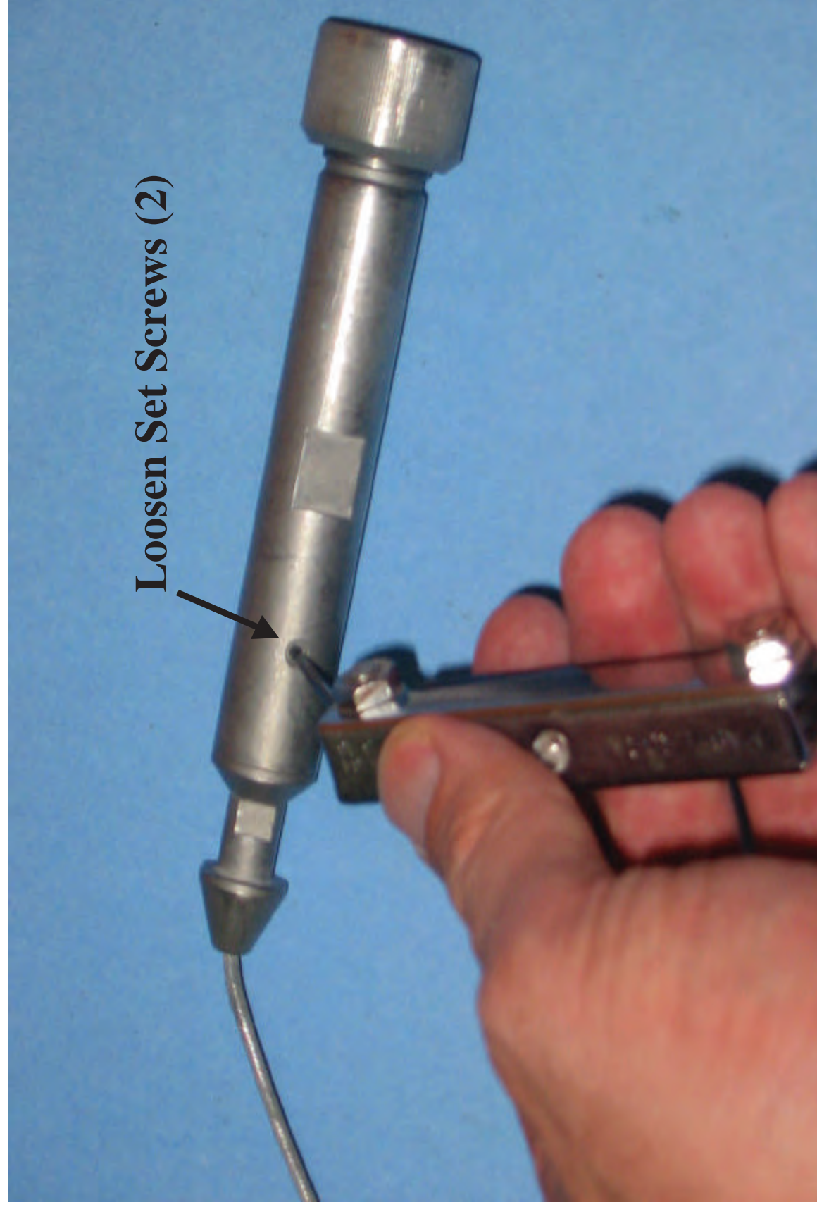
Pic.2 Cablehead Disassembly (1): Loosen set Screws
