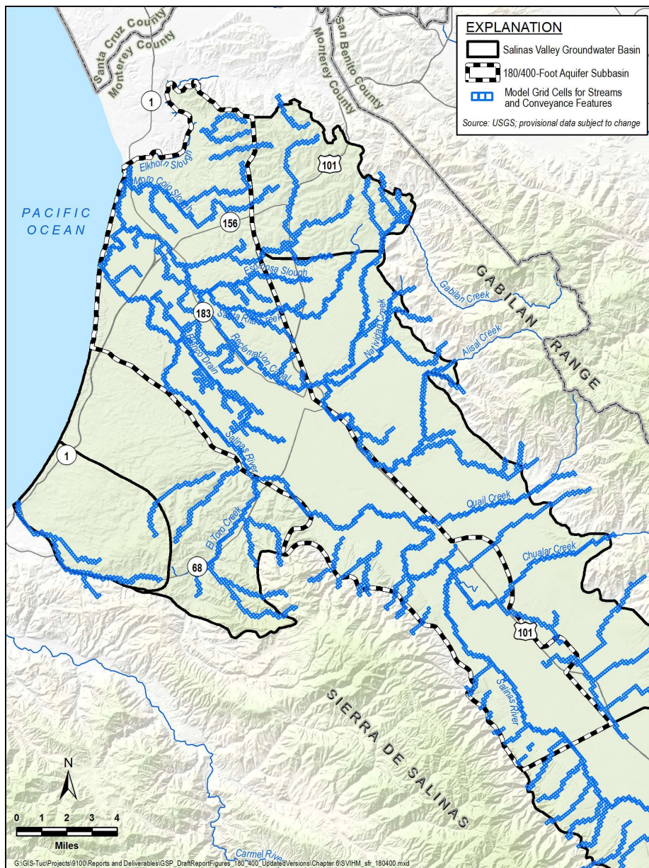
Figure 6-4. Surface Water Network in the 180/400-Foot Aquifer Subbasin from the Salinas Valley Integrated Hydrologic Model
