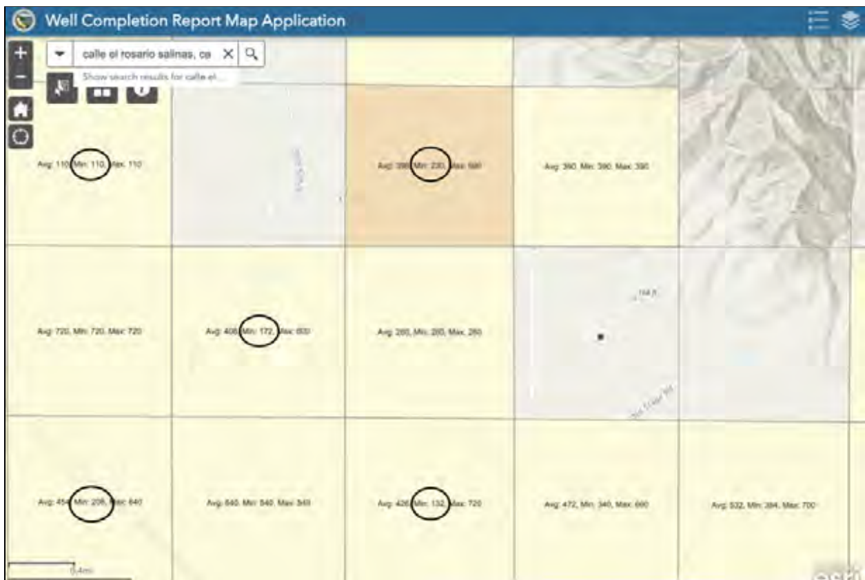
CWC Figure 10: Screenshot of DWR Well Completion Report Map application in the area near San Jerardo Cooperative highlighting that several 1 mi. by 1 mi. square sections include private domestic wells less than 250 feet deep.
