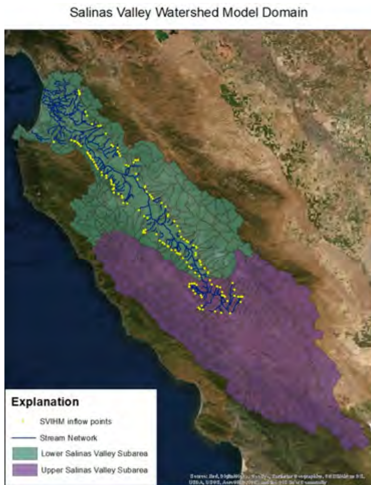
Figure 1: Salinas Valley Watershed Model (SVWM) domain showing Upper and Lower Salinas Valley Subareas, stream network, and inflow points where watershed flows are routed into the Salinas Valley Integrated Hydrologic Model (SVIHM).
