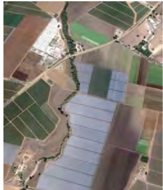
Figure 3 Gabilan creek above the City of Salinas with reduced of riparian and floodplain due to encroachment. Note opportunity areas along creek to reclaim lost floodplain while limiting loss of agriculture production.
