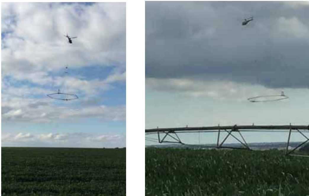
Figure 3-4: Photos of the SkyTEM312 system in suspension beneath the helicopter.
