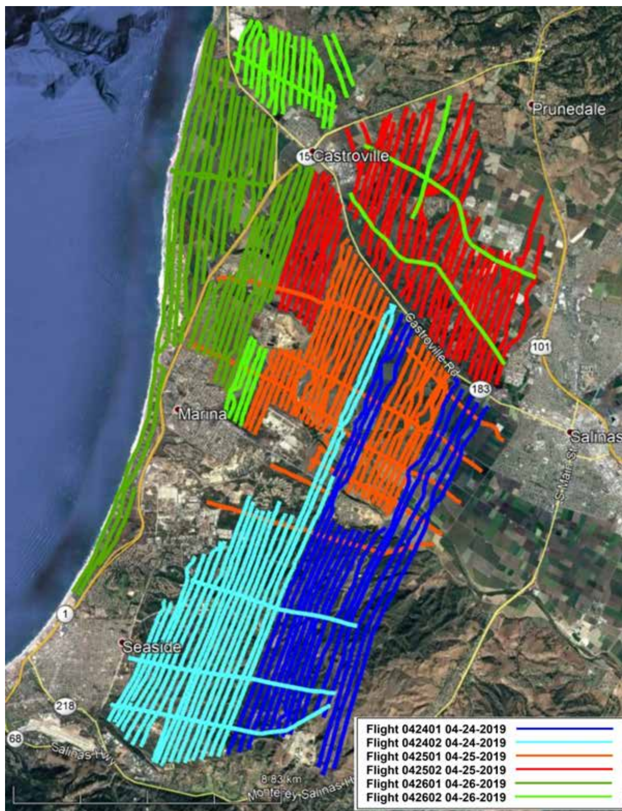
Figure 3-5: As-Flown map showing timing of the MCWD 2019 AEM survey data acquisition.
