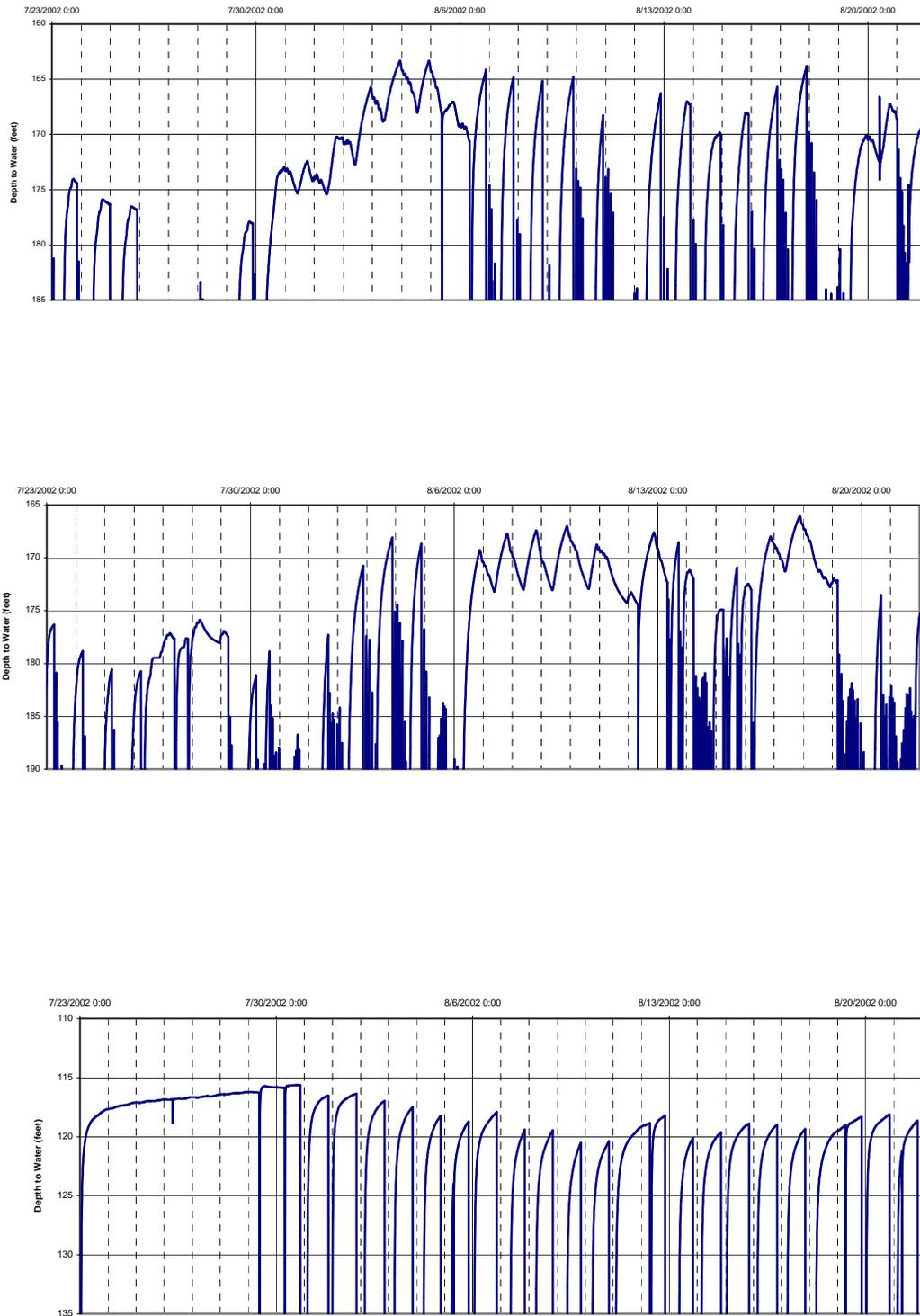
Figure 15. Well interference testing, MCWD wells 10, 11, and 12
