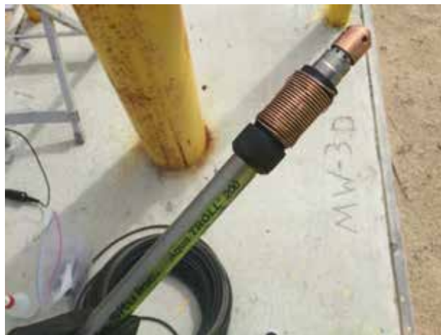
Figure 2-1. Downhole Water Level and Pressure Transducer
