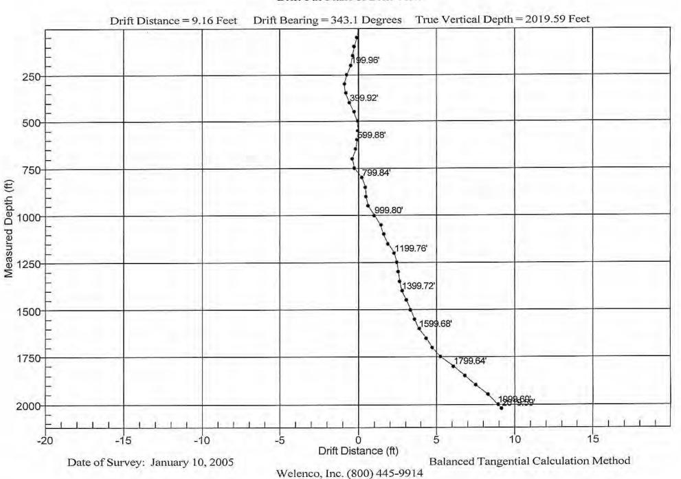
Deep Aquifer Test Well #1 Drift-Pac 3D Projection View
