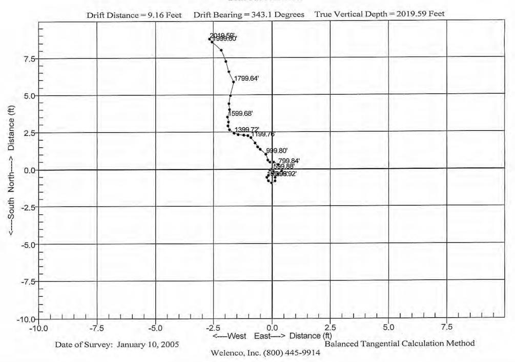
Deep Aquifer Test Well #1 Drift-Pac Plane of Drift View
